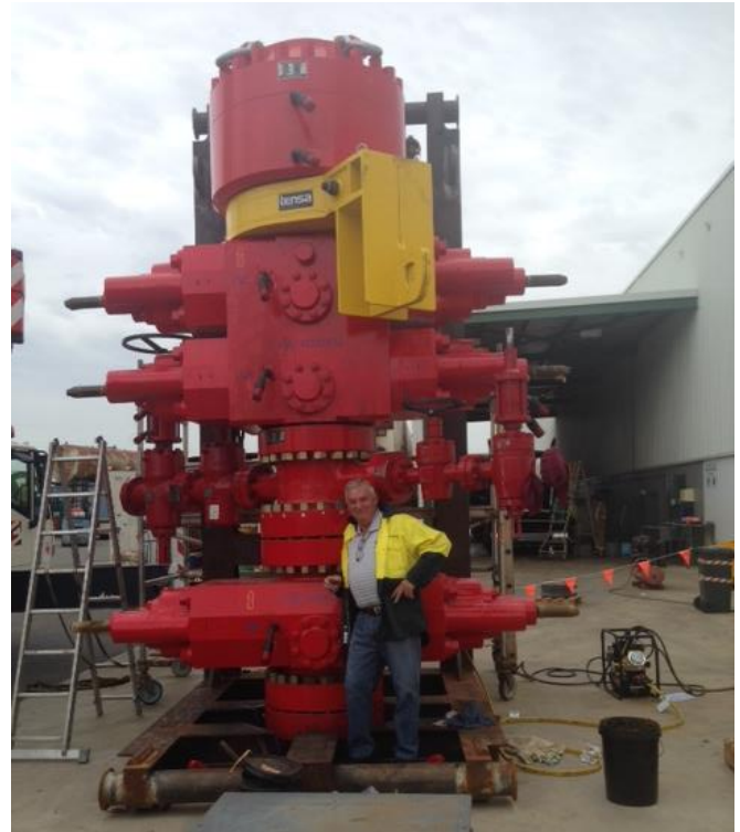
The new Blow Out Preventer (BOP)
